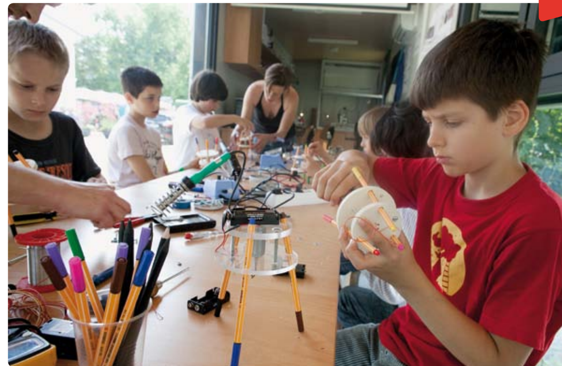
The drawing made by autonomous drawing dance of simple little robot that has pens as legs.
